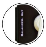
Balanced XLR output (200 ohm) for direct recording or PA (Not digital audio). PLEASE NOTE when using this output does the AUX input not work, nor the master volume. In this mode ONLY guitar the input, and amp/speaker simulator are active. The volume is set on the guitar knob, please be aware not overloading the mixing consol input.
