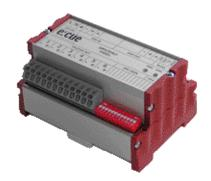
A flexible converter from DMX signal to DALI/DSI, DMX2DALI is a simple solution for controlling electrical DALI/DSI ballasts and dimmers using a DMX controller. DMX2DALI's flexibility makes installations easy by using auto and manual DMX addressing modes, and the option of using an RJ45 connector or loose wire for DMX connection.
