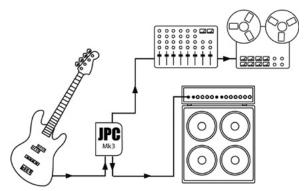
An instrument with active pickups connects to the 1/4" input. If a thru-put to an amp is required an adaptor must be applied to the like RCA output.
