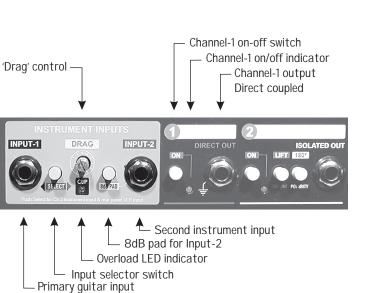
Input-2 is dual function. It is used for a second guitar and to access the rear XLR female input jack. This is a switching jack with front panel priority. When the front 1/4" input jack is used (has a jack connected), it becomes active. When it is not used, the rear XLR female input jack
