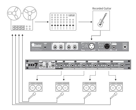
JD7 Instrument inputs, Channel-1 & Channel-2 outputs.
