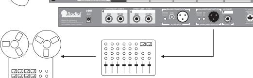
Replay the dry track, sending the signal to the XLR female input on the JD7. Select 'INPUT-2' by depressing the 'Select' switch on the front panel to turn on the XLR input. Adjust input level to suit. Now, play back the track through your amplifiers while trying different settings. This way, you can monitor different sounds before committing final track to tape.
