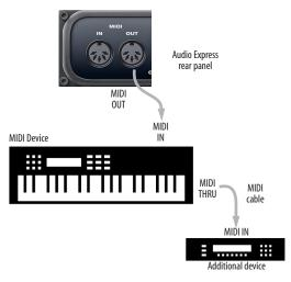
Figure 3-4: Connecting additional devices with MIDI THRU ports.
