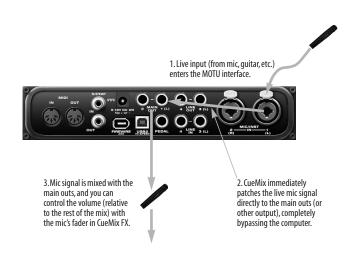
Figure 10-2: This diagram shows the signal flow when using CueMix no-latency monitoring. Notice that this method does not process the live input with plug-ins in your audio software.
