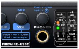
Figure 6-4: The Mix LEDs indicate which mix you are controlling with the front panel.
