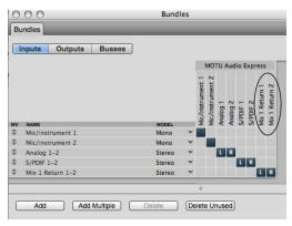
Figure 8-2: The Mix1 stereo return from the Audio Express in AudioDesk's Bundles window can be used to feed the Audio Express output back into AudioDesk.
