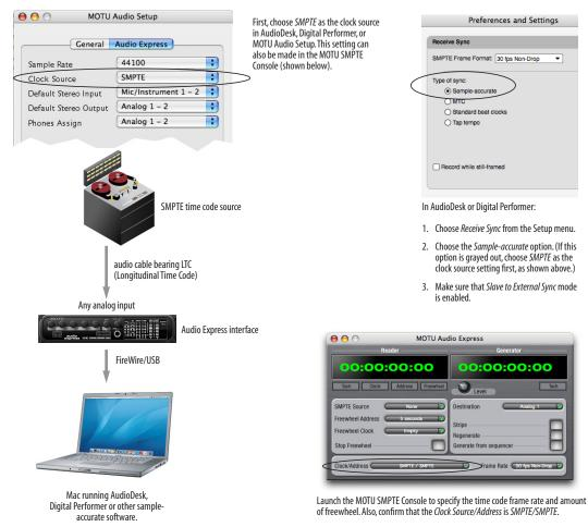
Figure 12-3: Connections for synchronizing the Audio Express directly to SMPTE time code.
