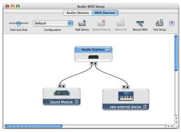
Figure 4-3: Connecting devices to the Audio Express. In this example, a controller keyboard is connected to the Audio Express's MIDI IN, and a sound module is connected to the Audio Express MIDI OUT.
