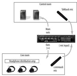
Figure 11-2: Typical hardware setup for Talkback and Listenback.
