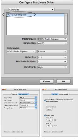
Figure 8-1: Choose Setup menu> Configure Audio System> Configure Hardware Driver to open the dialog shown above and access the Audio Express Core Audio driver. To access the rest of the Audio Express settings, open MOTU Audio Setup.
