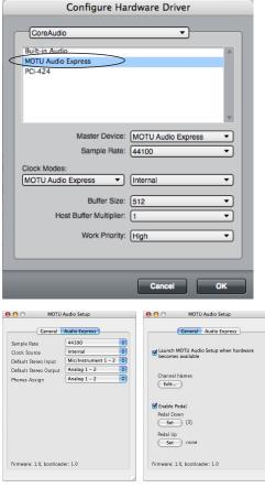
Figure 7-1: Choose Setup menu> Configure Audio System> Configure Hardware Driver to open the dialog shown above and access the Audio Express Core Audio driver. To access the rest of the Audio Express settings, open MOTU Audio Setup.
