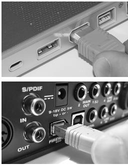
Figure 3-1: Connecting the Audio Express to the computer via FireWire.
