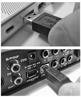
Figure 3-2: Connecting the Audio Express to the computer via USB.
