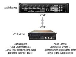
Figure 3-5: The setup for synchronizing a S/PDIF device with the Audio Express. Sync is achieved via the digital I/O connection itself. In this case, you have to choose S/PDIF as the Audio Express's clock source when resolving it to the other device.
