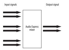
Figure 6-3: The Audio Express mixer takes all the input signals and combines them to an output. You control the volume of each input separately to produce a good mix.
