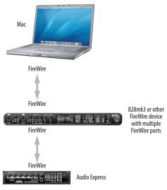
Figure 3-8: Connecting multiple MOTU FireWire audio interfaces.
