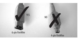
Figure 3-6: 4-pin FireWire connectors cannot be used for bus power.
