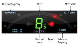
The *Tuner* window is an accurate and easy to use tuner.
