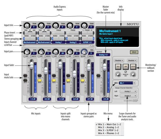
Figure 10-1: CueMix FX is a virtual mixer that gives you control over the Audio Express's on-board mixing features.
