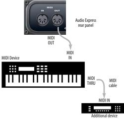
Figure 4-4: Connecting additional devices with MIDI THRU ports.
