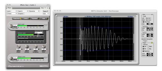
Figure 10-16: Viewing transients in the Oscilloscope
