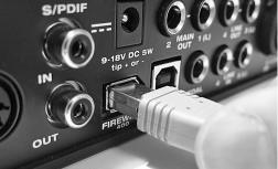
Figure 4-1: Connecting the Audio Express to the computer via FireWire.
