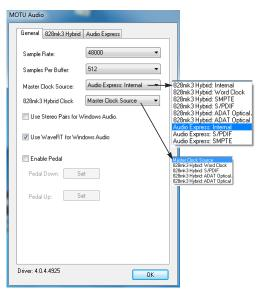
Figure 4-10: Choosing clock sources with multiple interfaces.
