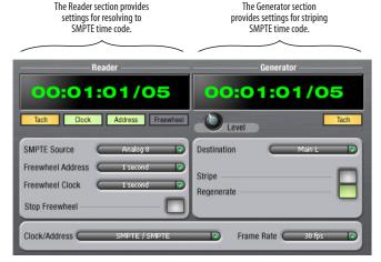
Figure 11-1: SMPTE Setup gives you access to your Audio Express's on-board SMPTE time code synchronization features.
