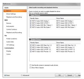
Figure 8-3: Activating the MOTU Audio WDM driver in SONAR by highlighting Audio Express inputs and outputs.
