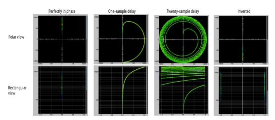
Figure 10-30: Two identical audio streams in the Phase Analysis.
