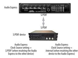
Figure 4-5: The setup for synchronizing a S/PDIF device with the Audio Express. Sync is achieved via the digital I/O connection itself. In this case, you have to choose S/PDIF as the Audio Express's clock source when resolving it to the other device.
