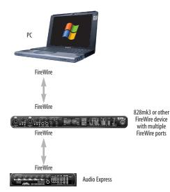
Figure 4-8: Connecting multiple MOTU FireWire audio interfaces.
