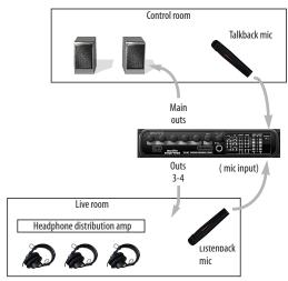
Figure 10-2: Typical hardware setup for Talkback and Listenback.
