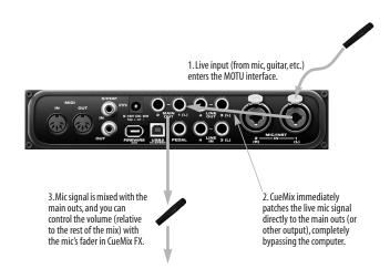
Figure 9-2: This diagram shows the signal flow when using CueMix no-latency monitoring. Notice that this method does not process the live input with plug-ins in your audio software.
