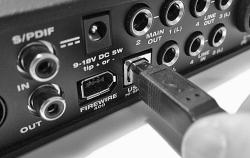
Figure 4-2: Connecting the Audio Express to the computer via USB.
