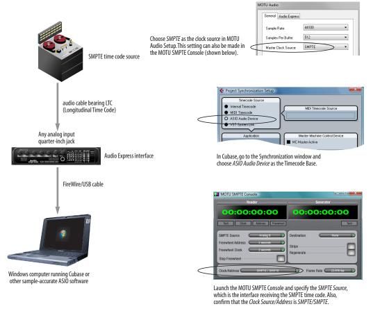
Figure 11-3: Connections for synchronizing the Audio Express directly to SMPTE time code.
