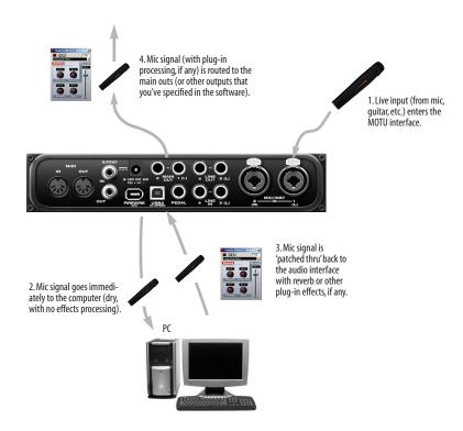
Figure 9-1: There are two ways to monitor live audio inputs with an Audio Express: 1) through the computer or 2) via CueMix hardware monitoring. This diagram shows method 1 (through the computer). When using this method, use your host software's buffer setting to reduce the slight delay you hear when monitoring the live input, but don't lower it too much, or your computer might get sluggish.
