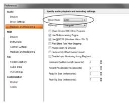
Figure 8-4: Enabling the ASIO driver instead of the WDM driver.
