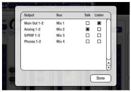
Figure 10-4: Routing the Talkback and Listenback mics to outputs.
