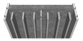
If the vertical deflectors are to be fixed in place insert a second metal pin in the rear hole of each deflector. Skip this step if the deflectors are to be movable and continue to step-8.
