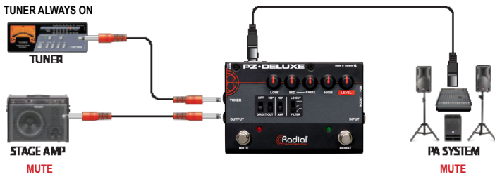
Depressing the MUTE footswitch turns off the 1/4" OUTPUT and the DI-OUT allowing for silent tuning or instrument changes.
