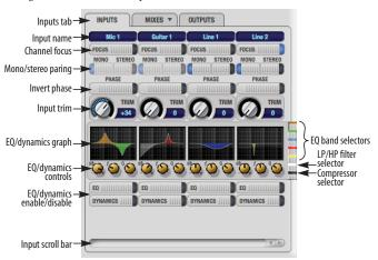
Figure 7-2: The Inputs tab.
