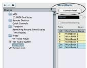
Figure 5-5: In Cubase or Nuendo, choose Devices menu> Device Setup and select the MicroBook to access the window above and the Audio Buffer Size setting (via the Control Panel button).
