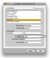
Figure 5-4:In Digital Performer and AudioDesk, choose Setup menu> Configure Audio System> Configure Hardware Driver to open the dialog shown above and access the Buffer Size setting. Refer to your Digital Performer or AudioDesk user guide for information about the Host Buffer Multiplier settina.
