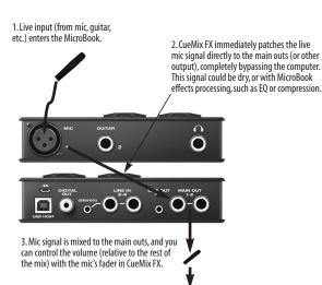
Figure 5-3: This diagram shows the signal flow when using CueMix FX no-latency monitoring. Notice that this method does not process the live input with plug-ins in your audio software. Instead, you can apply MicroBook effects, such as the EQ and/or compression.
