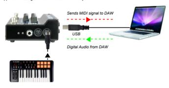
Application: Using a laptop as the MIDI source to control an external drum machine
