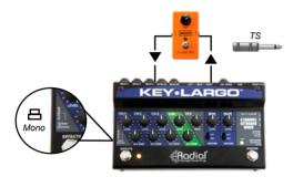
For stereo pedals and effects, make sure that the recessed Effects switch is disengaged. Use insert cables wired with 1/4" TRS to 1/4" TRS to 1/4" TRS connectors to connect the SEND jack to the left and right inputs of the effects unit, and use a second insert cable to connect the outputs of the device to the TRS RECV connector on the Key-Largo.
