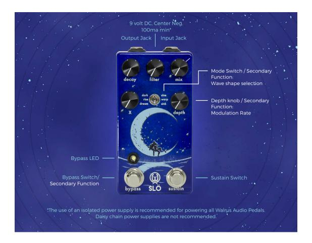
DECAY - Adjusts the length of the reverb decay. Go from tight short reverb, at full counter-clockwise, to long drawn out texture at full clockwise.
