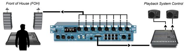
**XLR OUTPUTS:** The front panel XLR outputs feaure DI box transformers that provide isolation to eliminate hum and buzz from ground loops when connecting to distant PA systems. Individual ground lift switches are also provided on each channel to further eliminate noise.
