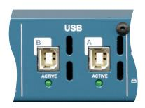
**ACTIVE** LEDs indicate connection to each computer
