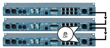
Linking multiple SW8-USB units using 1/4" TRS cables
