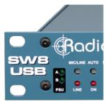
Front panel PSU A and B indicators
