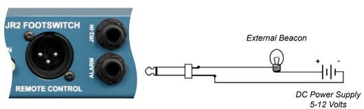
Using the ALARM output to trigger an external device
