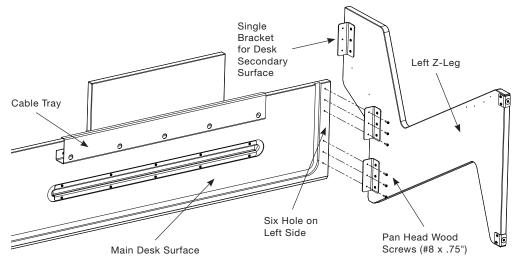
Stand up main desk surface with cable tray at the top. Stand up left z-leg, making sure the single bracket for the desk secondary surface is at the top. Line up the two brackets on the left z-leg with the six holes on the left side of the main desk surface. Use pan head wood screws (#8 X .75") to attach left z-leg to main desk surface. Repeat this with the right z-leg
