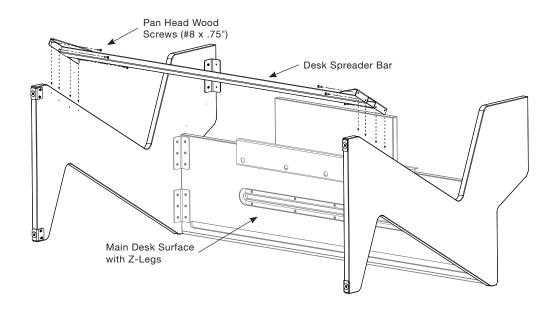
While the desk is still laying down, attach desk spreader bar to both z-legs. Line up spreader bar with z-leg holes. Use 4 pan head wood screws (#8 X .75") on each side.
