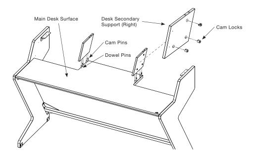
Slide the desk secondary supports onto the dowel rods and cam pins.
