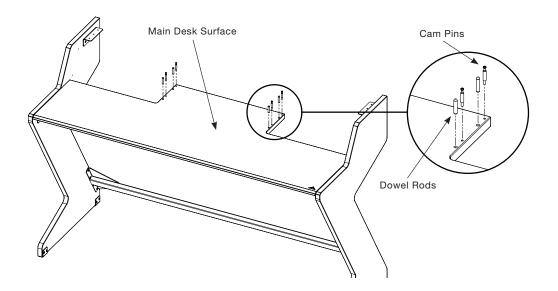
On the back end of the main desk surface find the small holes and screw in cam pins. In the larger holes push in dowel rods.
