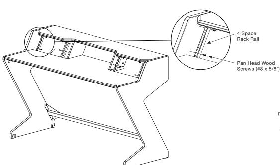
In the two side gaps between the main and secondary desk surfaces, screw in the rack rails (4 Space) on either side. Use the shorter pan head wood screws (#8 X 5/8") to attach.
