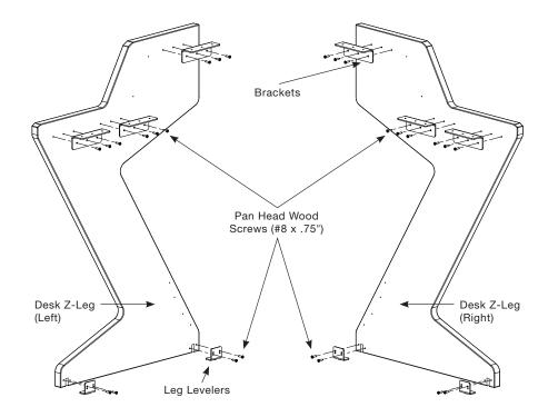
Lay both Z-legs down with holes facing up. Attach three brackets to each of the z-legs. Use three pan head wood screws (#8 x 75") for each bracket. At the base of each z-leg attach leg levelers. Use two pan head screws (#8 x 75") for each of the leg levelers.
