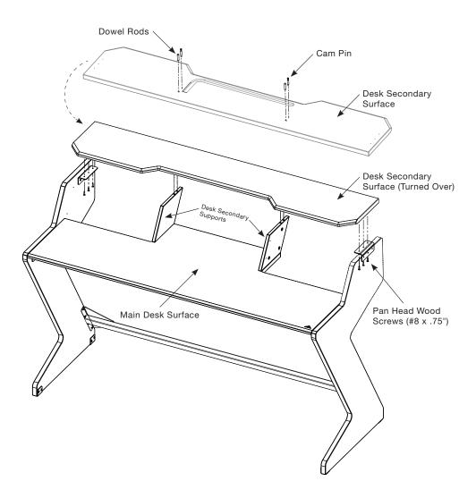
Lay the desk secondary surface on it's back. Groove and holes should be facing up. Find the small holes and screw in cam pins. In the larger holes push in dowel rods.
