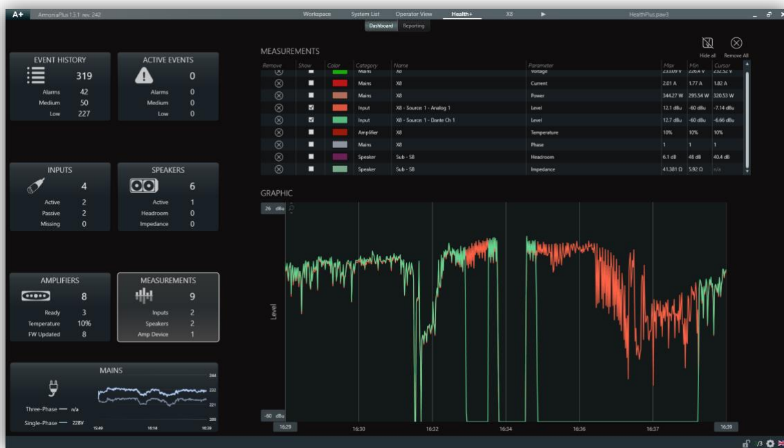
Figure 6 - Measurements Inputs: Dante and Analog in Backup Strategy.
