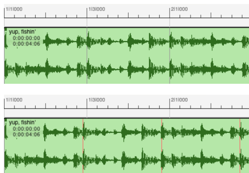
Figure 53-2: A soundbite recorded at 120 bpm in a 120bpm sequence (above), and the same soundbite placed in a 114 bpm sequence (below). Notice how the grid lines inside the soundbite no longer line up with the grid lines in the ruler to alert you to the fact that the soundbite tempo map doesn’t currently match the sequence’s tempo.
