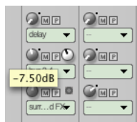
Figure 71-13: Send level is displayed as shown here as you adjust the send knob.
