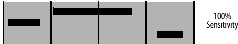
Figure 49-17: 100% Sensitivity reaches all the way from one grid location to the next, as shown here by the gray background.
