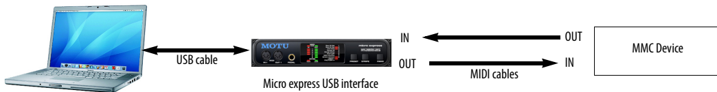
Figure 90-1: If the MMC device can generate MIDI Time Code (MTC), the MIDI connections shown here are all that are necessary. Be sure the MIDI interface internally routes the MTC to the computer.
