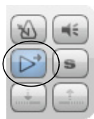
Figure 23-5: Enabling and disabling Auto Scroll by window type using the Auto Scroll button in the Control Panel.
