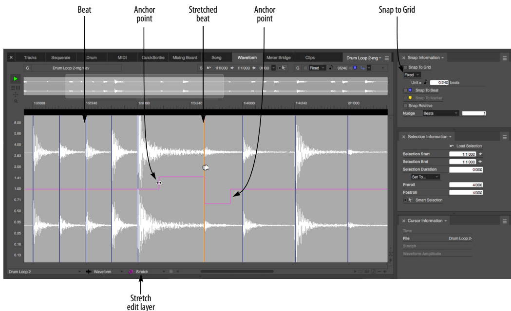
Figure 54-9: The Stretch layer in the Waveform Editor. The Snap to Grid setting determines the anchor points surrounding the beat you drag.
