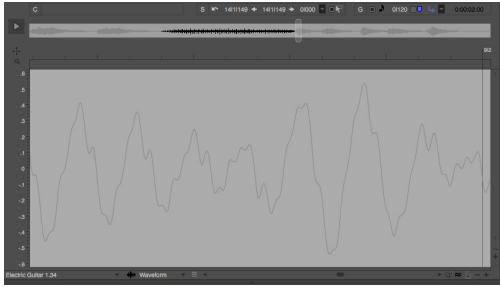
Figure 45-4: The Waveform Editor can zoom in to the sample level. Zooming in this far makes it easy to make precise edits on individual samples.
