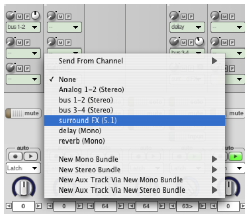
Figure 71-12: In this example, the send is being assigned to a 5.1 surround bus.
