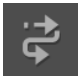
Figure 68-6: The Chain Chunks button makes Digital Performer cue up and start playing the next sequence or song in the Chunks window when it reaches the end of the current one.
