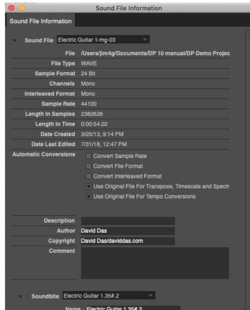
Figure 7-24: In the Automatic Conversions section, check items to enable them. These settings override the settings in the Automatic Conversions preferences.
