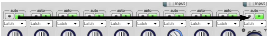
Figure 71-27: Gliding across the Solo, Mute, and automation play buttons. You can combine gliding with the Command/Ctrl and Option/Alt key modifiers as described in the table above.
