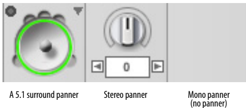
Figure 14-4: The output bundle assigned to a track determines what type of panner it has in the Mixing Board.
