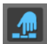
Figure 22-23: The Wait button causes Digital Performer to wait for an incoming MIDI event before it begins to play or record.
