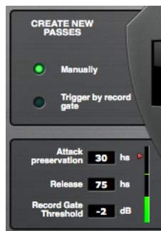
Figure 31-3: New passes can be created manually or automatically with the record gate.
