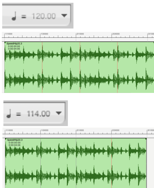
Figure 53-7: In this example, a 114 bpm Drum Loop has been placed in a new sequence set to 120 bpm as shown by the tempo indication (above). After selecting the soundbite and choosing Adjust Sequence to Soundbite Tempo , the tempo slider now exactly matches the tempo of the soundbite, as indicated by the time ruler grid lines, which now match up (below).
